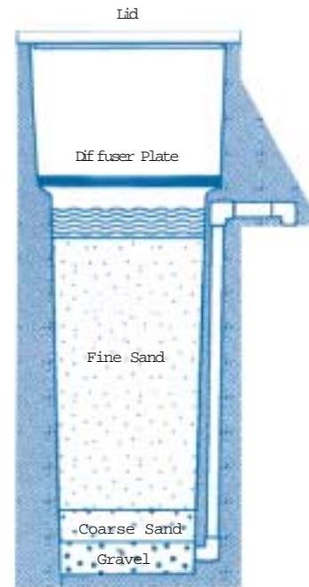
*Diagram of a water filter*
